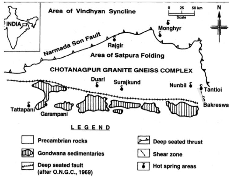
Figure 2. Regional geological setting of the geothermal areas in Eastern India.
