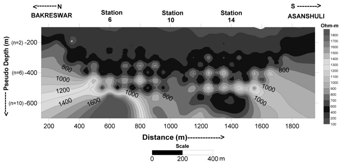
Figure 6. Collinear dipole-dipole resistivity profiling along Bakreswar-Asanshuli traverse.
