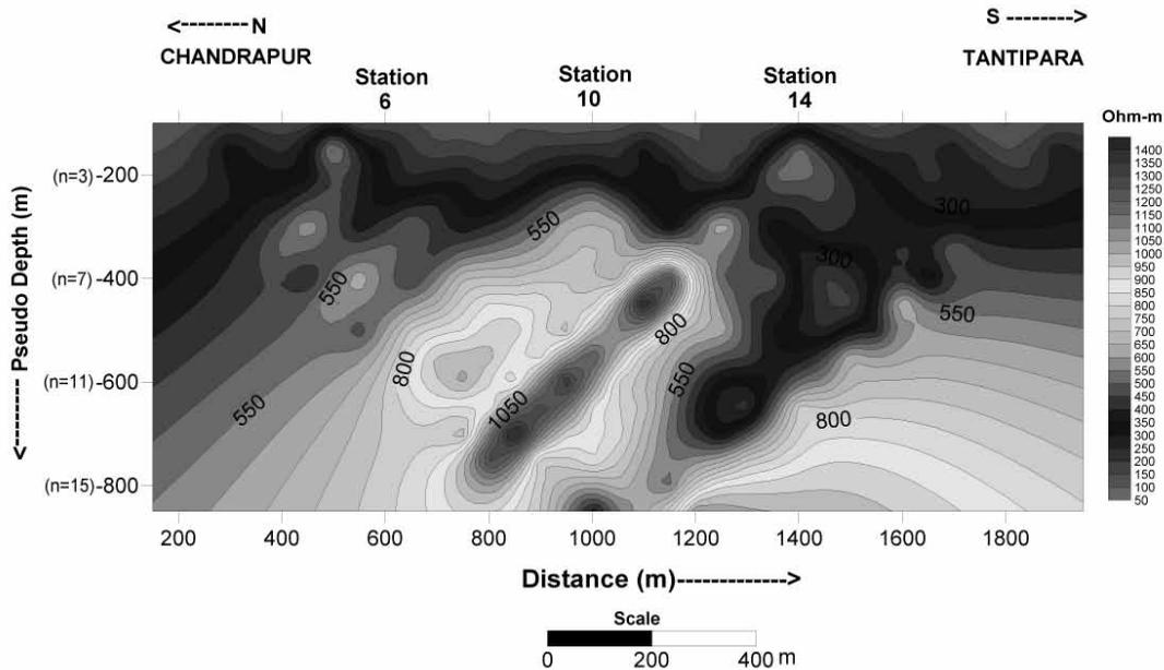
Figure 7. Collinear dipole-dipole profiling along Chandrapur-Tantipara traverse.
