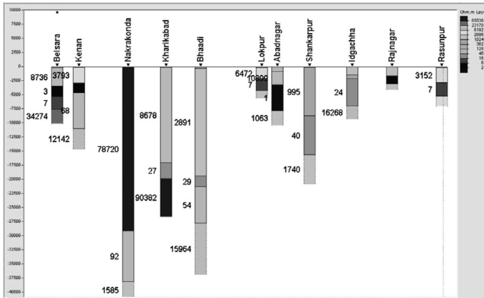
**Figure 4.** 1-D section along Belsara-Rajnar-Rasunpur traverse. Vertical scale: (Depth in m; Resistivity values in Ohm-m).
