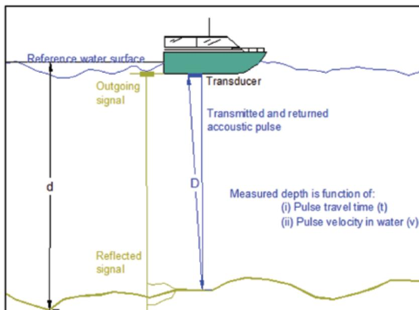
Figure 3. Schematic diagram showing principles of echo sounder.
